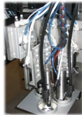
VALVES IN AUTOMATIC PURGE PROCESS
